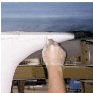
Fig. 13 The joint is tooled off and finished
