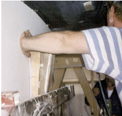
Fig. 11 A keel is carefully slid into position
