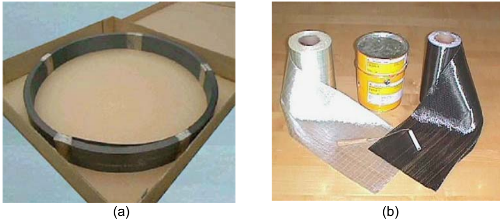
Fig. 4.1 Manufactured forms of FRP materials.
