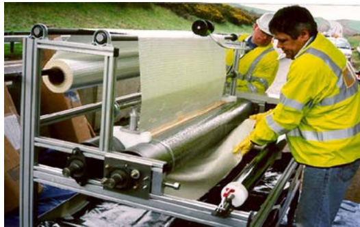
Fig 8.3 Saturator Machine for the SikaWrap “Wet” process.
